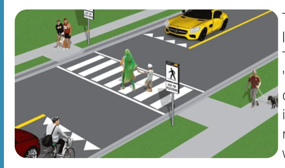
There are 4 types of PXO which are listed as type "A", "B", "C" or "D". The Township currently has type "C" and "D" pedestrian crossovers. The major difference between the two crossings is that a type "C" crossover has rectangular flashing beacons (RRFB) to warn motorists.
